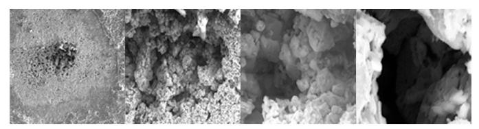
Analysis of the evaporator tube by a scanning electron microscope shows areas of intense micro-pitting consistent with biological attack. Pitting in this situation has resulted in tube wall losses of greater than 40% in an 8 year old chiller.
